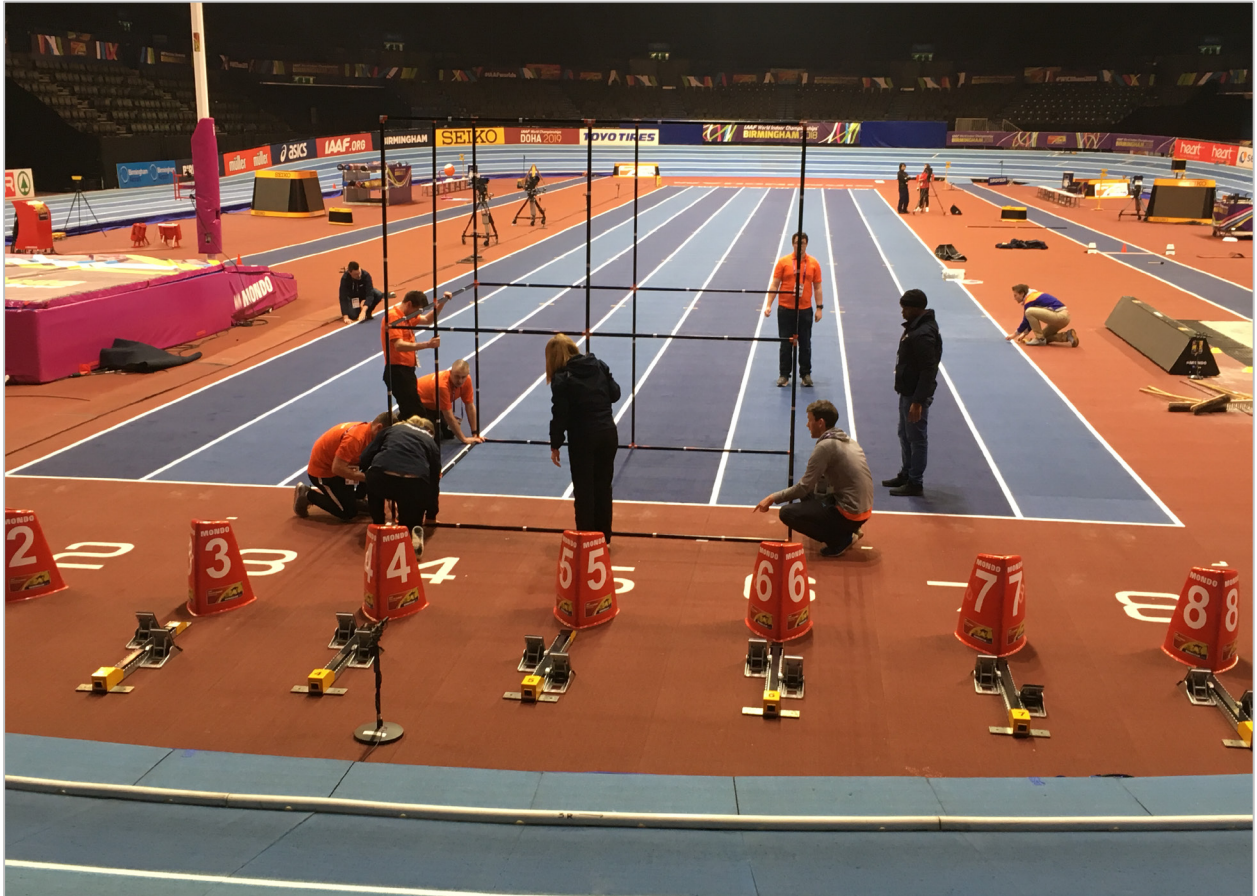
Figure 2. The calibration frame was constructed and filmed before and after the competition.
