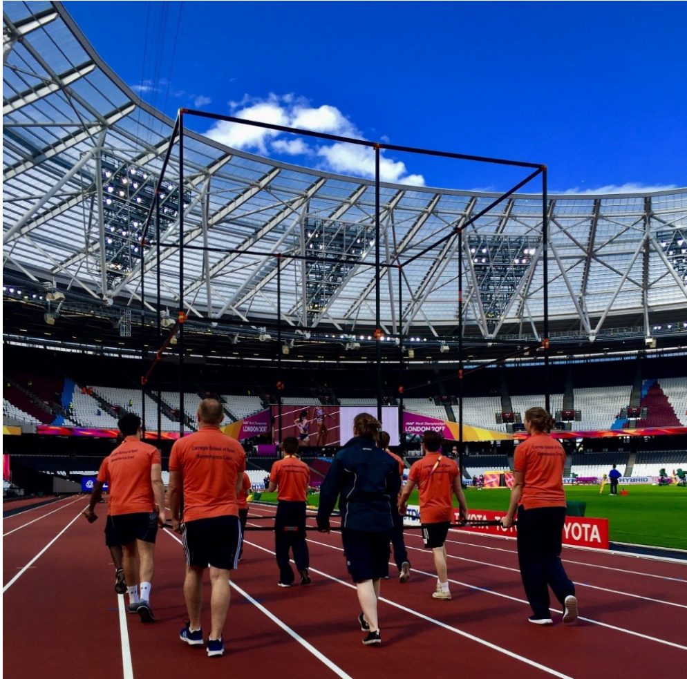
Figure 2. The calibration frame was constructed and filmed before and after the competition.
