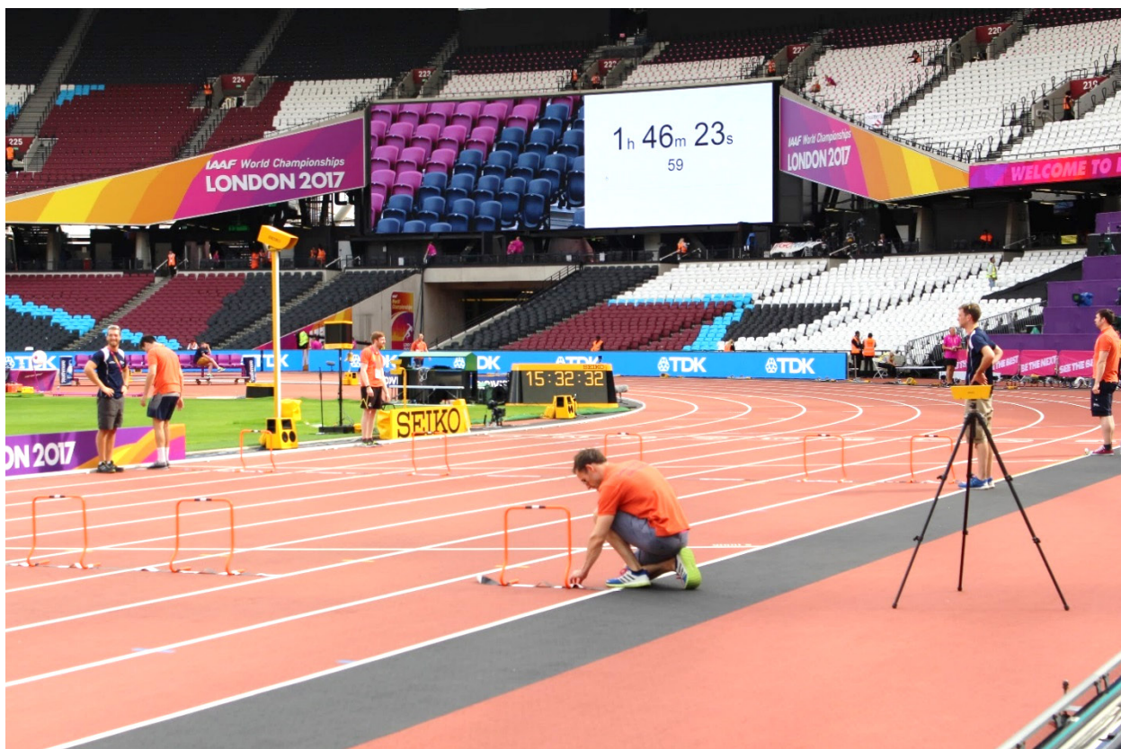
Figure 2. Set-up of the hurdle calibration system used to determine split intervals.
