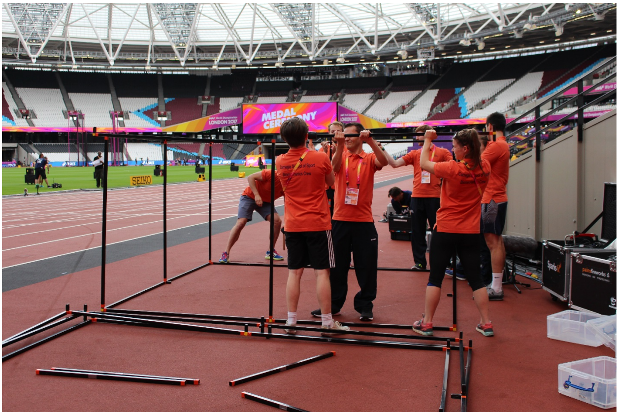
Figure 2. The calibration frame was constructed and recorded before and after the competition.
