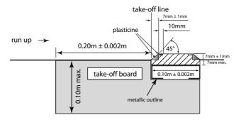
Figure 184a- Take-off board and plasticine indicator board
