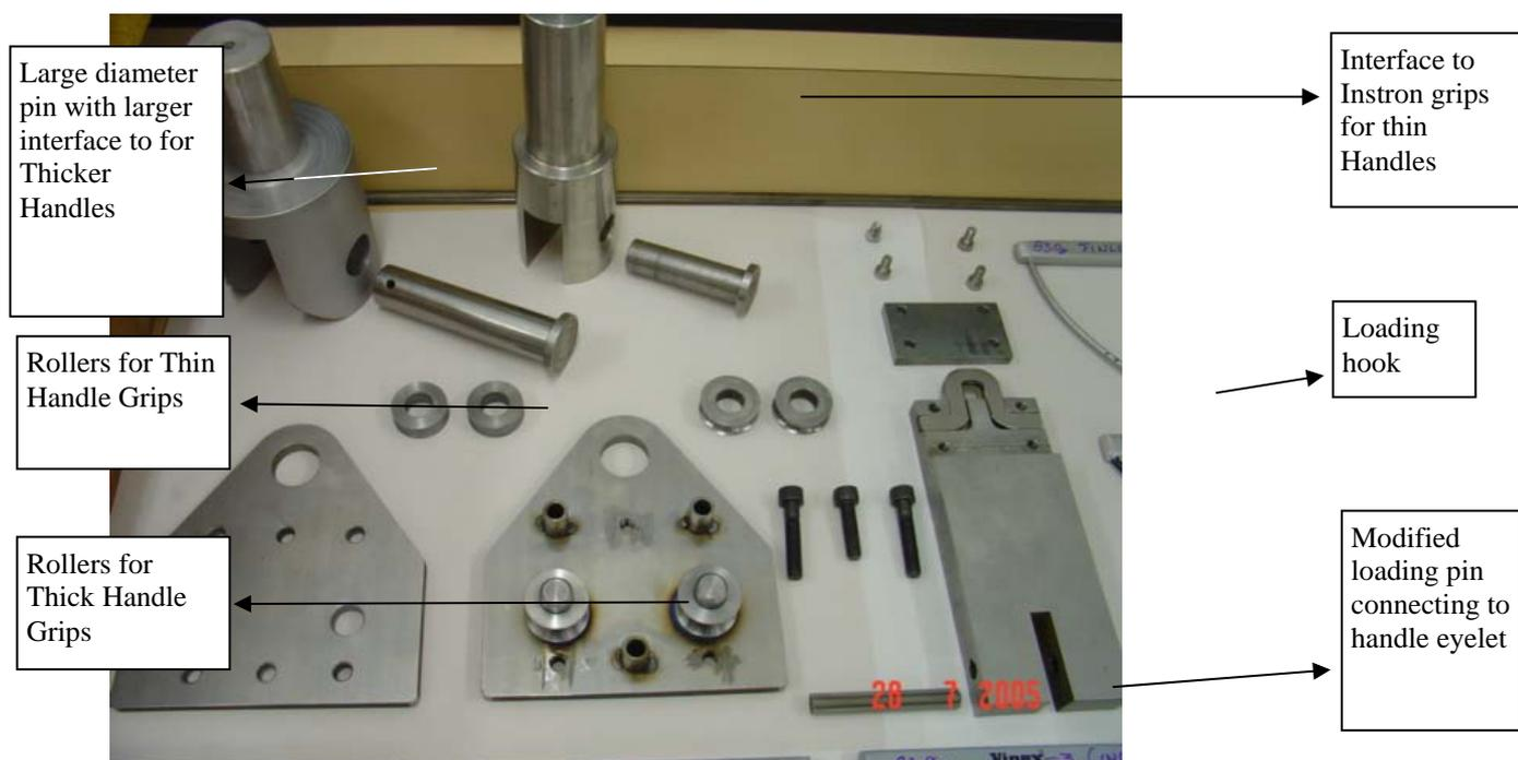
**Figure 2. Components of Modified Test Fixture**
