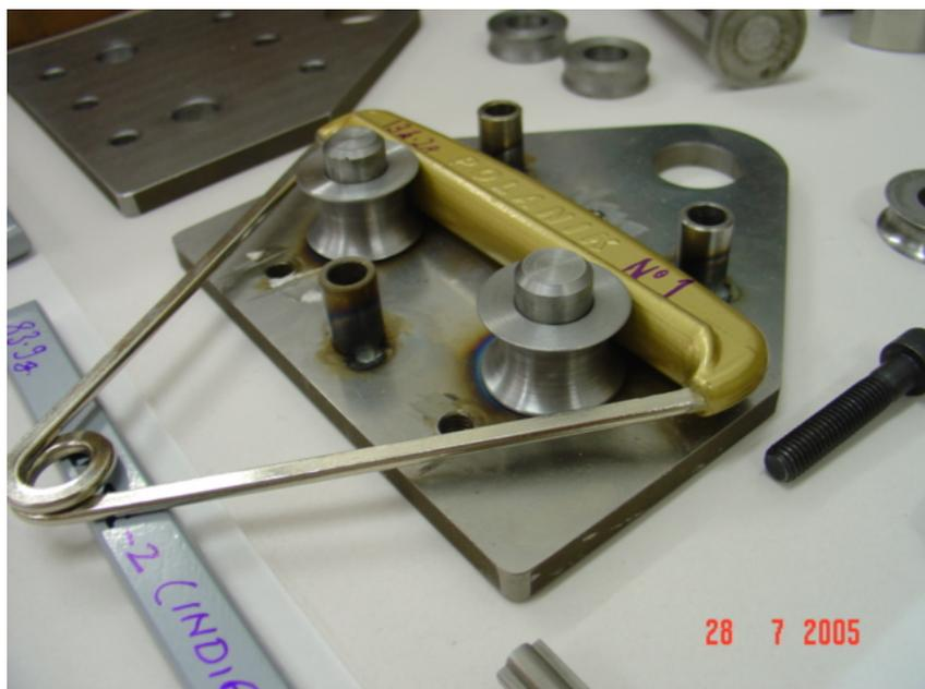
**Figure 3. Handle in the Modified Test Fixture
