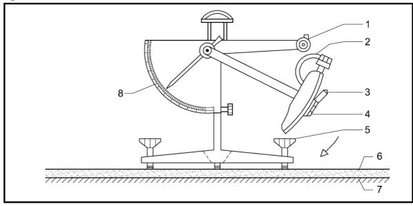
Figure 1 - Portable Skid Resistance Tester (Friction Method A)
