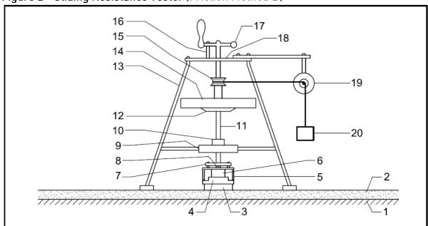
Figure 2 - Sliding Resistance Tester (Friction Method B)
