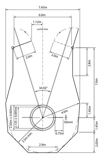
**Figure 22 - Cage for Hammer and Discus Throw with concentric circles** (Hammer Throw configuration)
