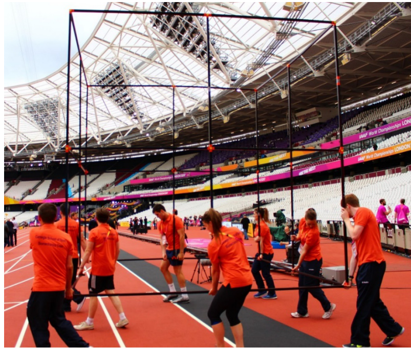
Figure 2. The calibration frame was constructed and recorded before and after the competition.
