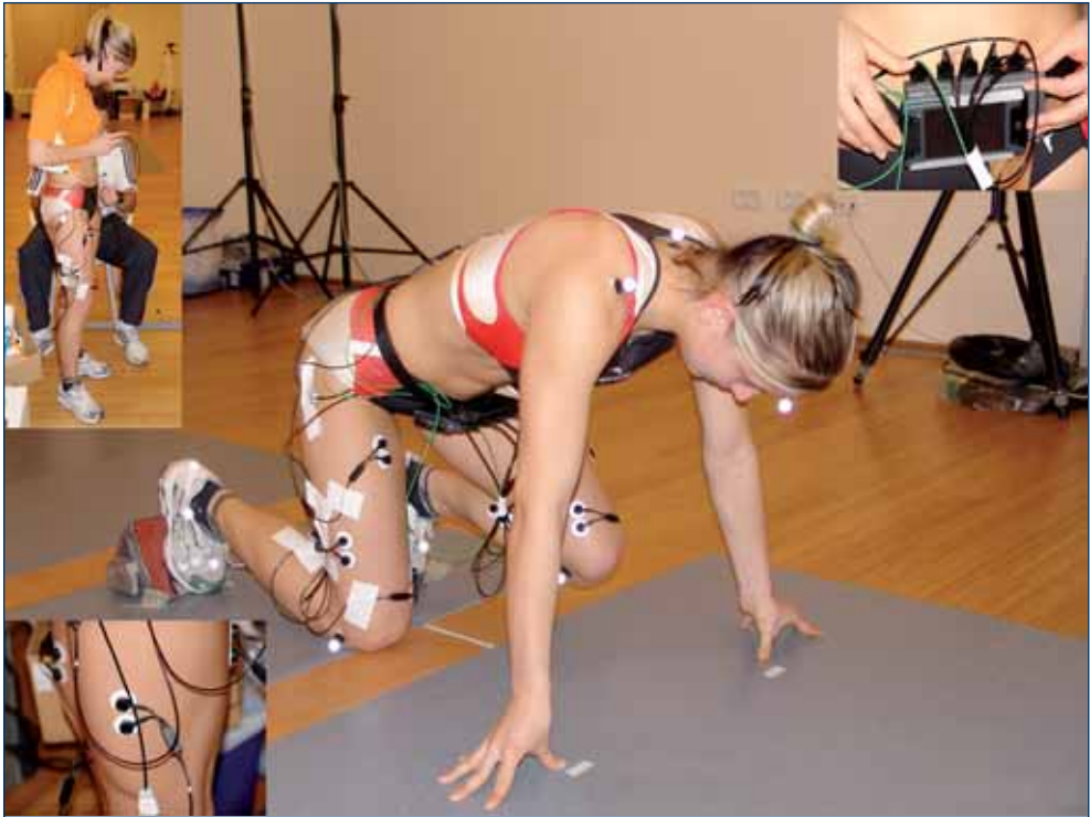
Figure 3: Placement of surface electrodes for measuring EMG activity
